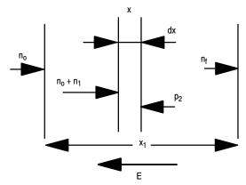
(b) Carriers pair are created in the region dx at x, by electrons flowing from the left and hole flowing from the right
