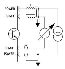
The values of R and L are adjusted for a given transistor and test conditions. Typical values are R=470  $\Omega$  and L=100  $\mu$ H. All the network must be located as close as possible to the transistor under test. Kelvin contacts are mandatory. Shielding cables are recommended.
