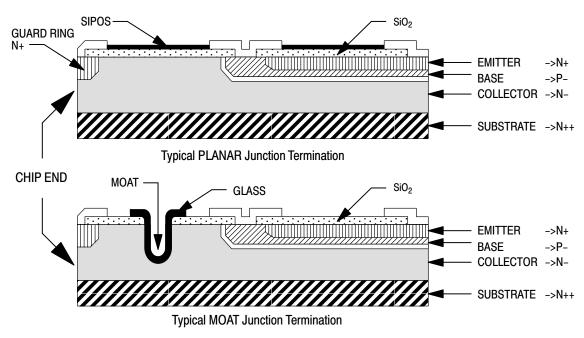
Figure 7. Typical Junction Terminations for a High Voltage Bipolar Transistor
