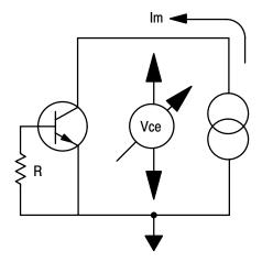
BVCES: reverse Collector to Emitter voltage, the Base shorted to the Emitter, under a given Collector current bias.
