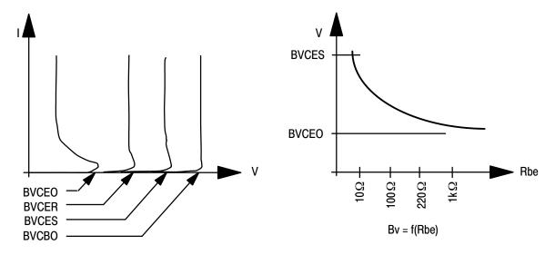
Figure 14. Typical Breakdown Curves (BVEBO not shown)
