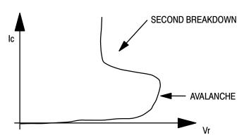
Figure 4. Typical Second Breakdown Characteristic
