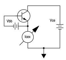
ICEY: Collector to Emitter current under reverse Collector to Emitter voltage, with a forward Base to Emitter bias.
