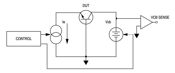
Figure 10. Typical Forward Bias Safe Operating Area Test Circuit
